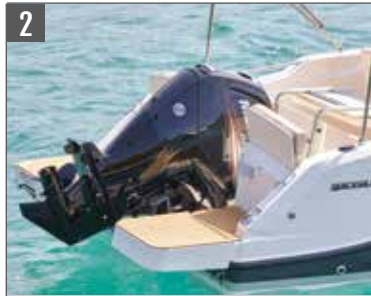
Reclining center backrest to allow full tilt engine position and maximal cockpit space
