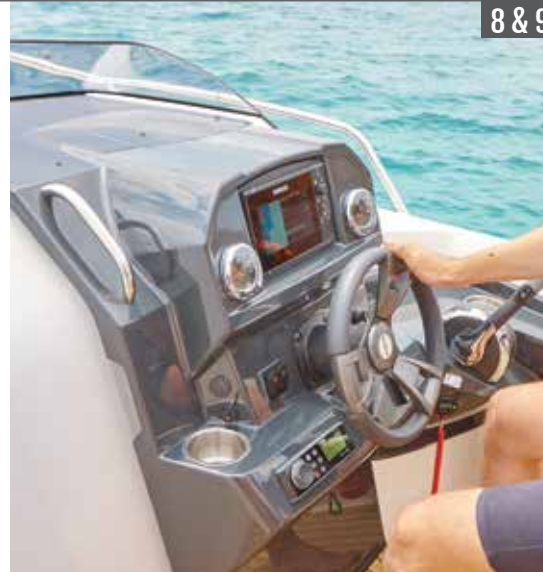
Helm with room for a 7" GPS/Chart plotter and instrumentation. Ergonomic armrest and cup holder
