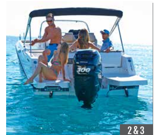
Double swim platforms. Motor well bridge: easy access to both sides of transom
